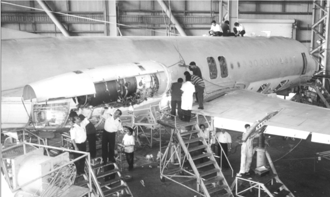
Photo shows Biman's engineers and technicians performing D-check on an F-28 aircraft in the Biman Engineering Hanger Complex at Kurmitola in the city. This is the second time Biman's engineers and technicians are carrying out D-checks on its F-28 aircraft which will save a huge amount in foreign exchange.
