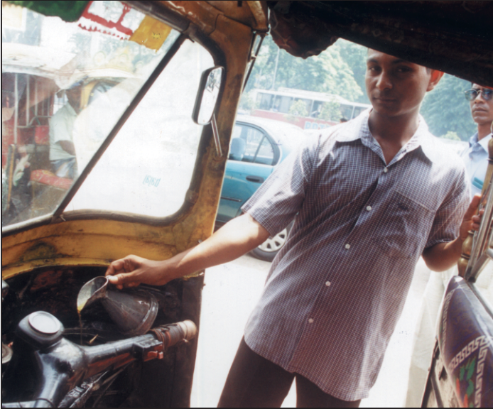
An auto-rickshaw driver pours engine oil into the petrol tank at a filling station in the city. When combusted, admixture of engine oil and petrol results in black smoke and causes severe air pollution.
