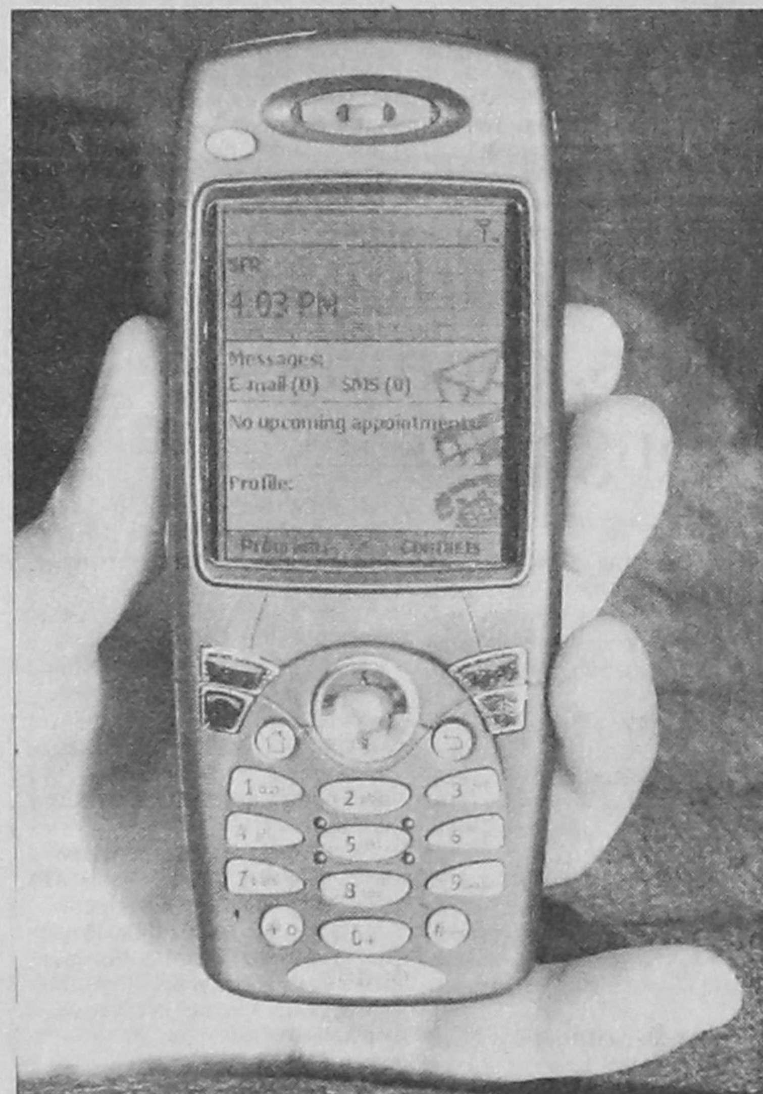
Shown is Sendo International's Z100 multimedia smartphone at a news conference during the GSM World Congress in Cannes, France, Wednesday. The Z100 phone features a colour screen and runs on the Microsoft smartphone platform. The phone also features Microsoft's Mobile Explorer for the Internet, Mobile Outlook, a Windows Media player and USB connectivity. The phone will be on the market in the autumn of 2001.
