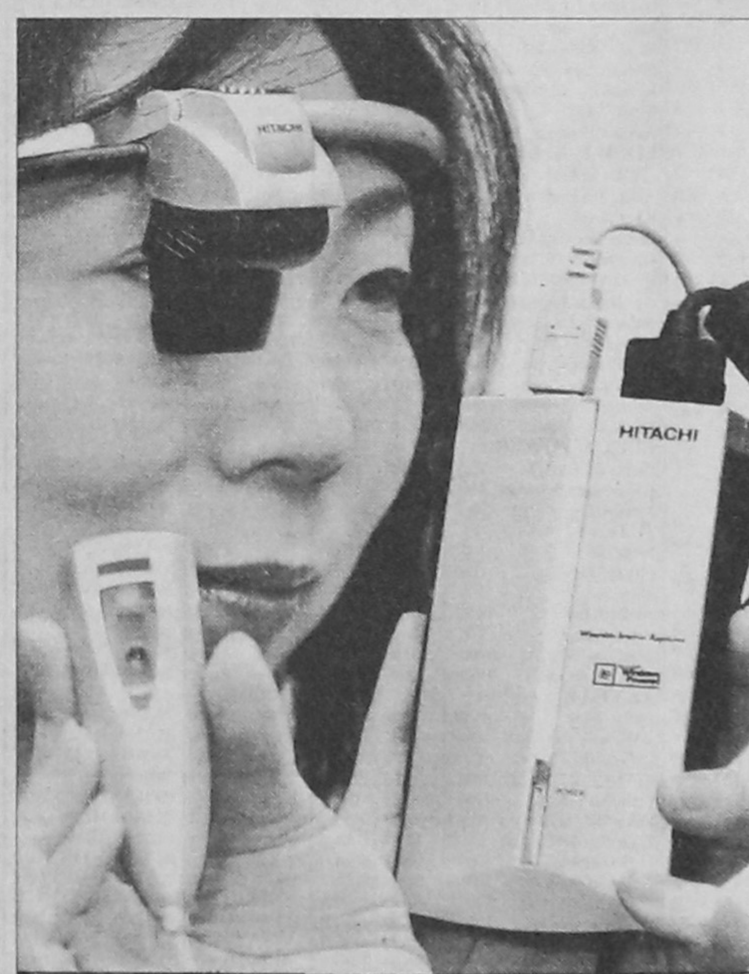
Japan's electronics giant Hitachi employee Masami Hasegawa displays a prototype of a wearable PC which consists of a palm-sized Windows CE based main unit weighing only 230 grams, a 70-gram HMD with a SVGA full-color LCD display and a pointing device in Tokyo yesterday. The wearable PC, produced by Hitachi, Shimadzu and Colorado MicroDisplay jointly, is expected to be placed on the world market this year with estimated price of 200,000 yen (1,700 USD).
