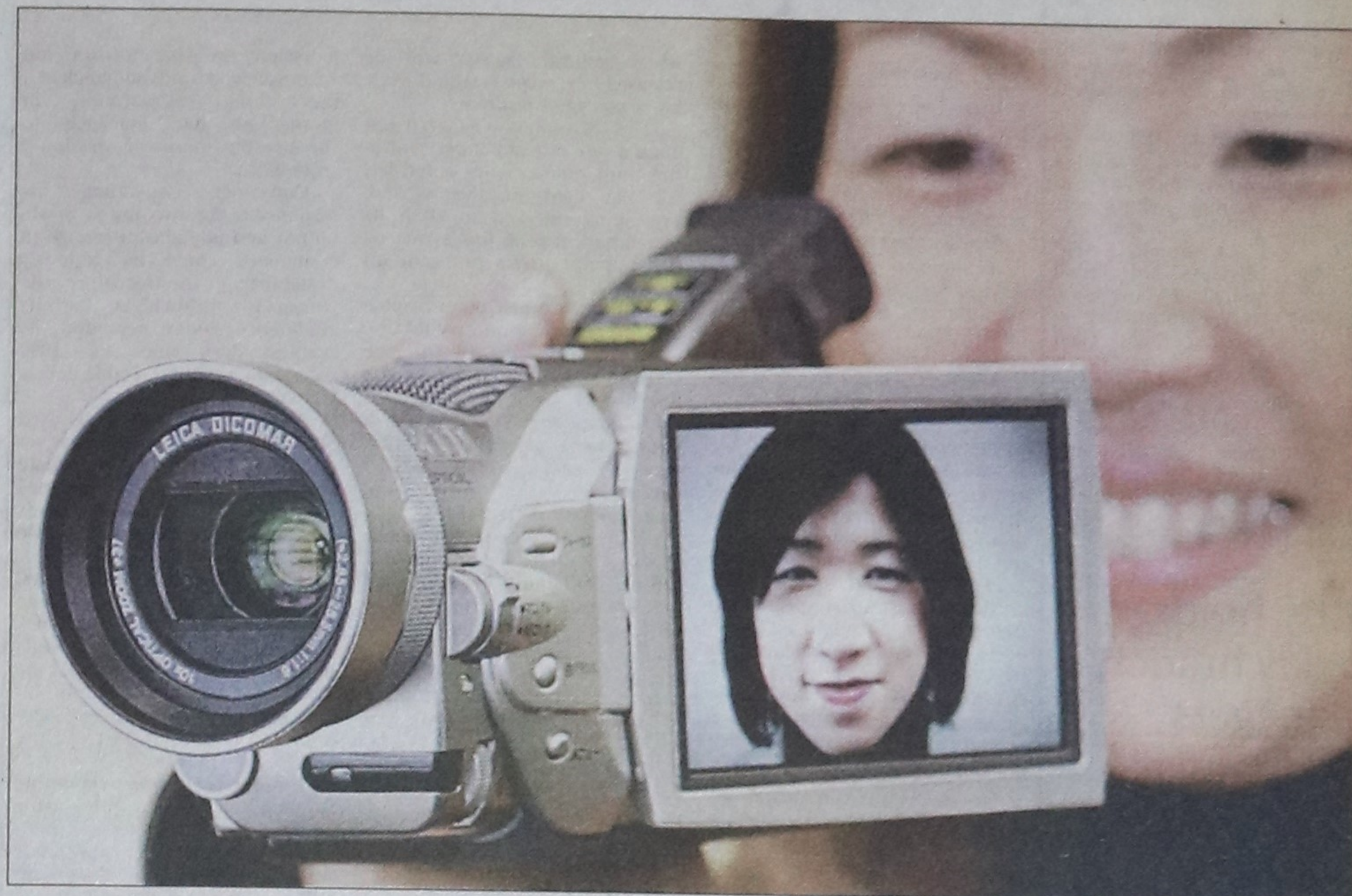
Japan's electronics giant Matsushita unveils the new 3-CCD digital video camcorder Digicam NV-MX2000 at the company's head office in Tokyo yesterday. The Digicam features a set of three 380,000-pixel CCDs on its image sensor and a 2.85-28.5mm/F1.6 Leica Digicam zoom lens equipped with an optical image stabiliser system. Matsushita will put it on the domestic market on February 1 with a price of 2,000 USD.
