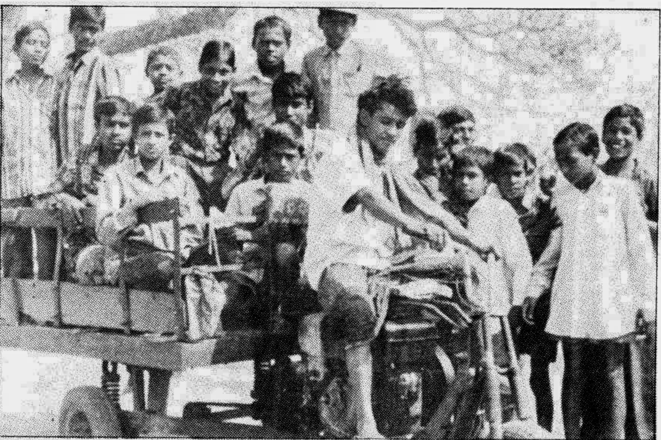
Multi-purpose machine: Shallow pumps originally meant for irrigation is now being used for mechanising surface transport after being used earlier for water transport. — Star photo
