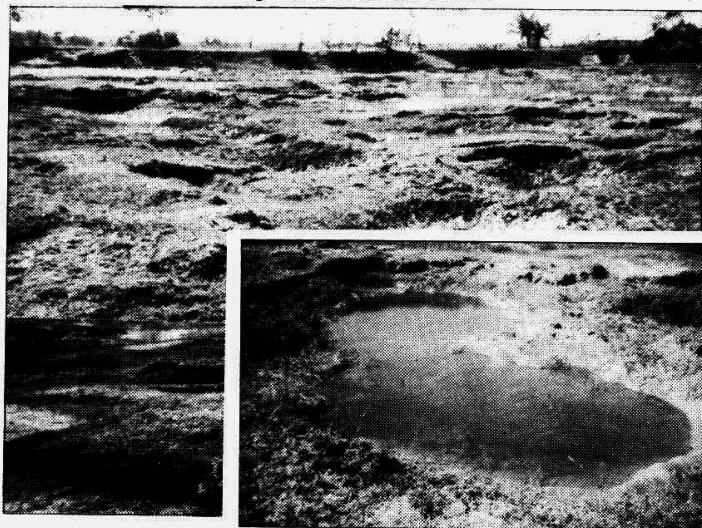
Crater formation on a plot after sand extraction and (inset) settlement trough formed under one borehole
