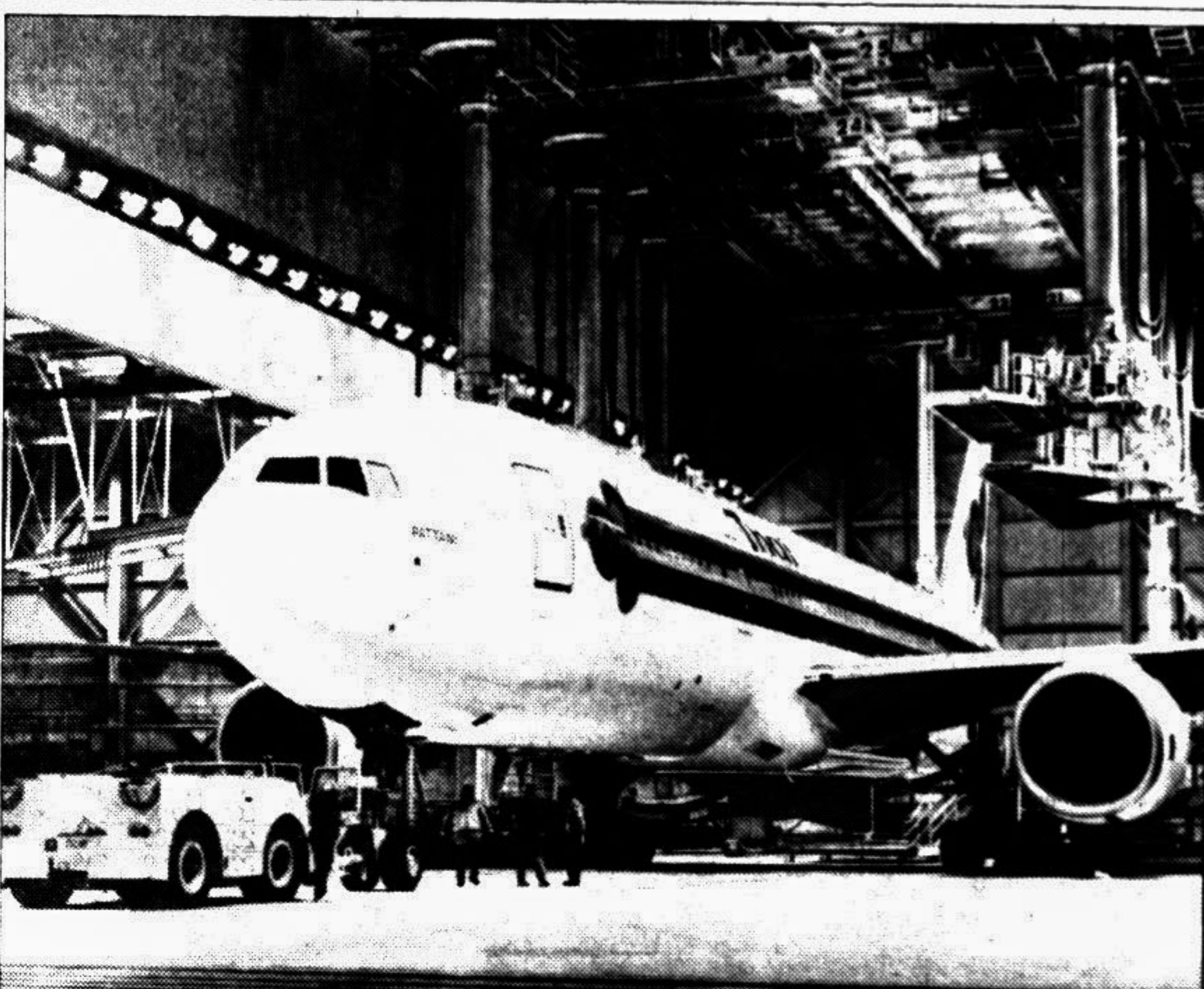
BOEING PAINTS 100TH 777 AIRPLANE: The 100th 777 built by Boeing rolled out of the company's paint hangar in Washington in Thai Airways' festive colours. The airplane, a-200 model, is the seventh of 14 777s ordered by the airline. This airplane required about 200 gallons of paint, which weighed approximately 600 pounds.
