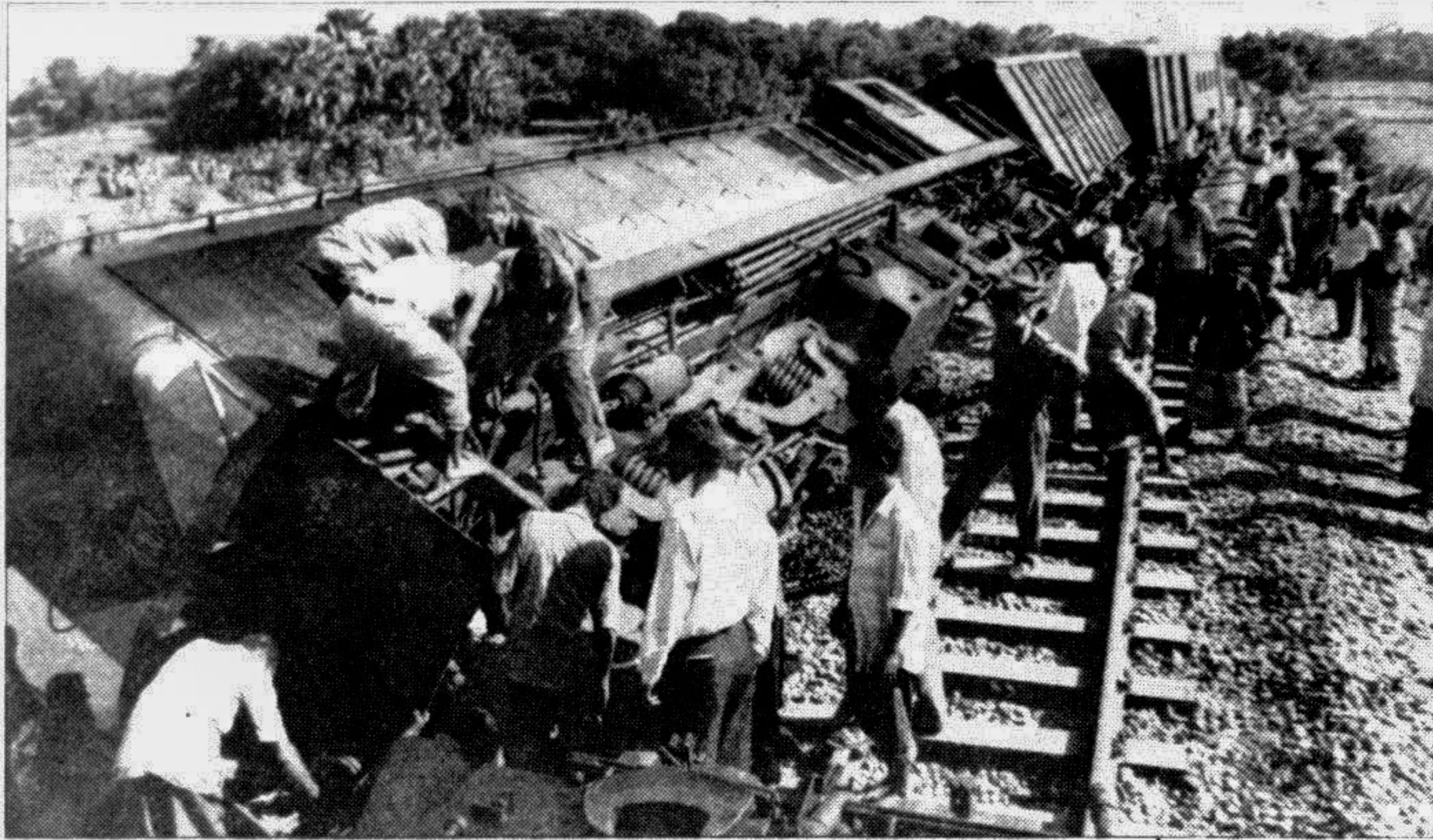
A Dhaka-bound train from Bhairab derailed at Nintali in Tongi in the early hours of yesterday as fish plates of the track were removed Sunday night to enforce the rail-road barricade. — Star photo
