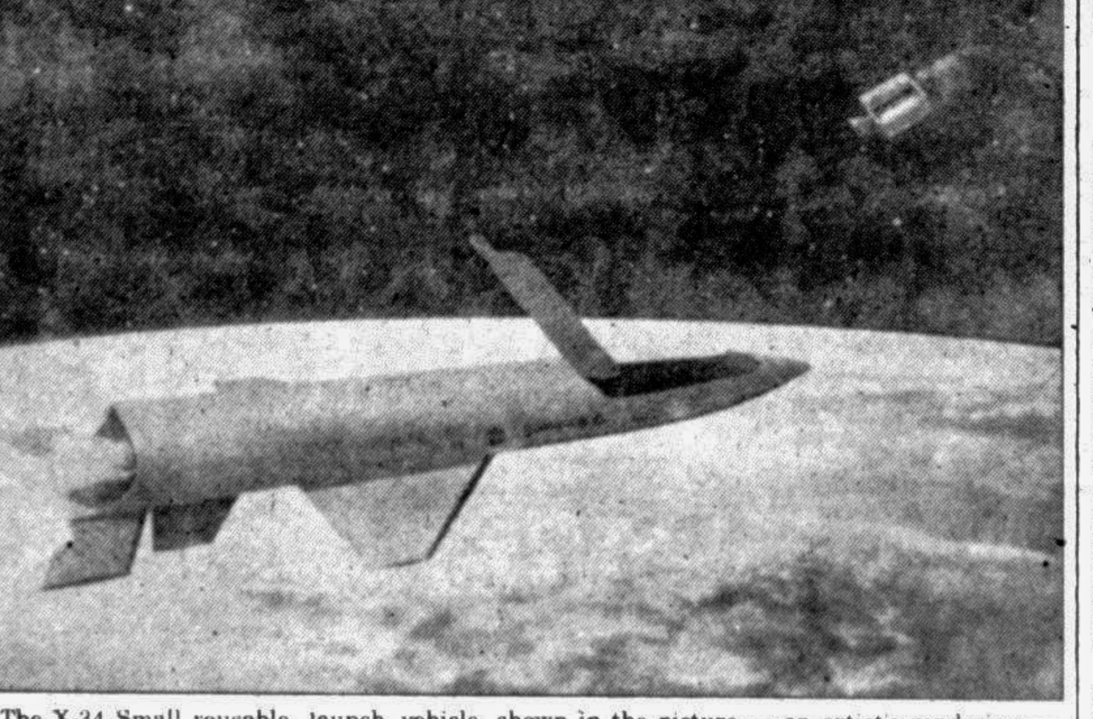
The X-34 Small reusable launch vehicle, shown in the picture — an artist's rendering — made available on Friday by Orbital Sciences Corporation, will release satellites in space, re-enter the atmosphere and land on a conventional runway. The launch vehicle is an unmanned alternative to the current space shuttle and will be developed cooperatively by Orbital Sciences Corporation, Rockwell International and NASA. — AFP/UNB photo
