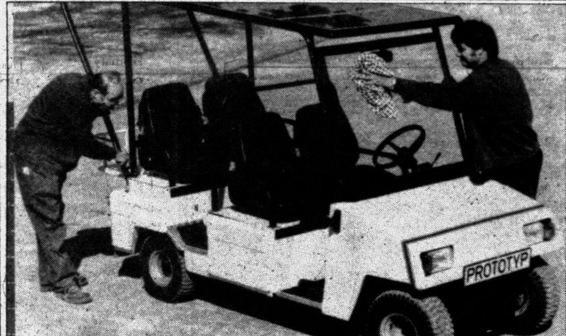
The prototype of a new solarmobile (Solar Nord GmbH, Wismar) from eastern Germany. The solar cells on the roof generate a 300-watt output for feeding the on-board batteries. The vehicle has a range of 40km (25 miles) with a top speed of 50 kph (31.25 mph). — IN photo
