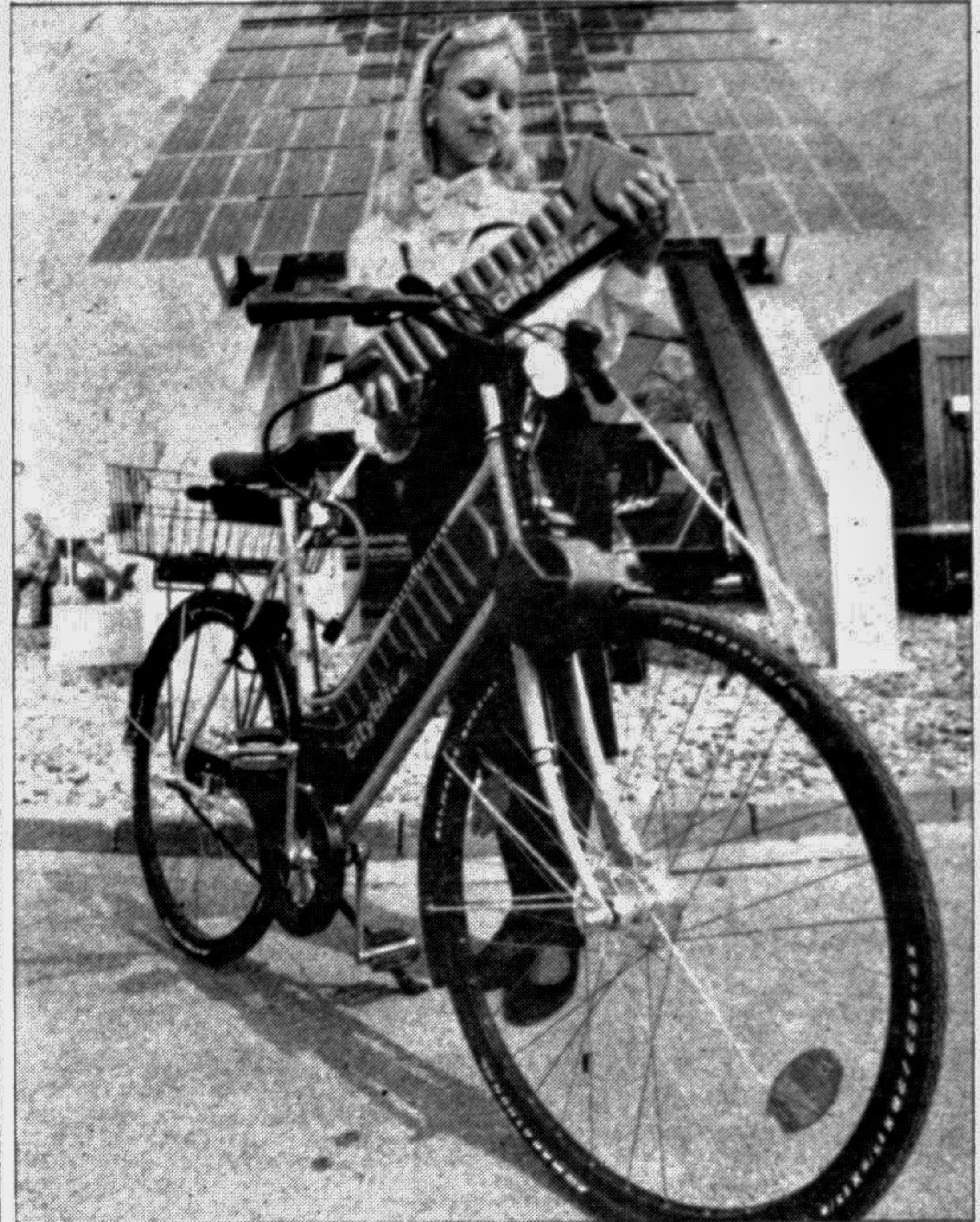
A hostess at the Hanover Fair shows a bicycle battery that can be recharged at a solar service station. The small power pack, attached to the crossbar, drives a front-wheel motor that saves burdensome pedalling for about one hour. — IN press photo
