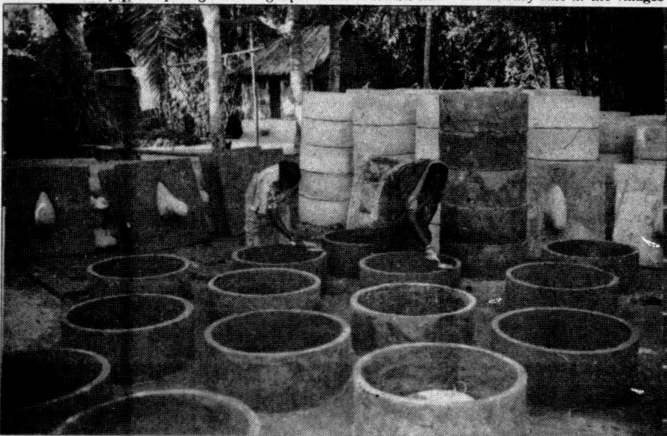
Women preparing concrete slab latrines — for sanitation and income generation.
