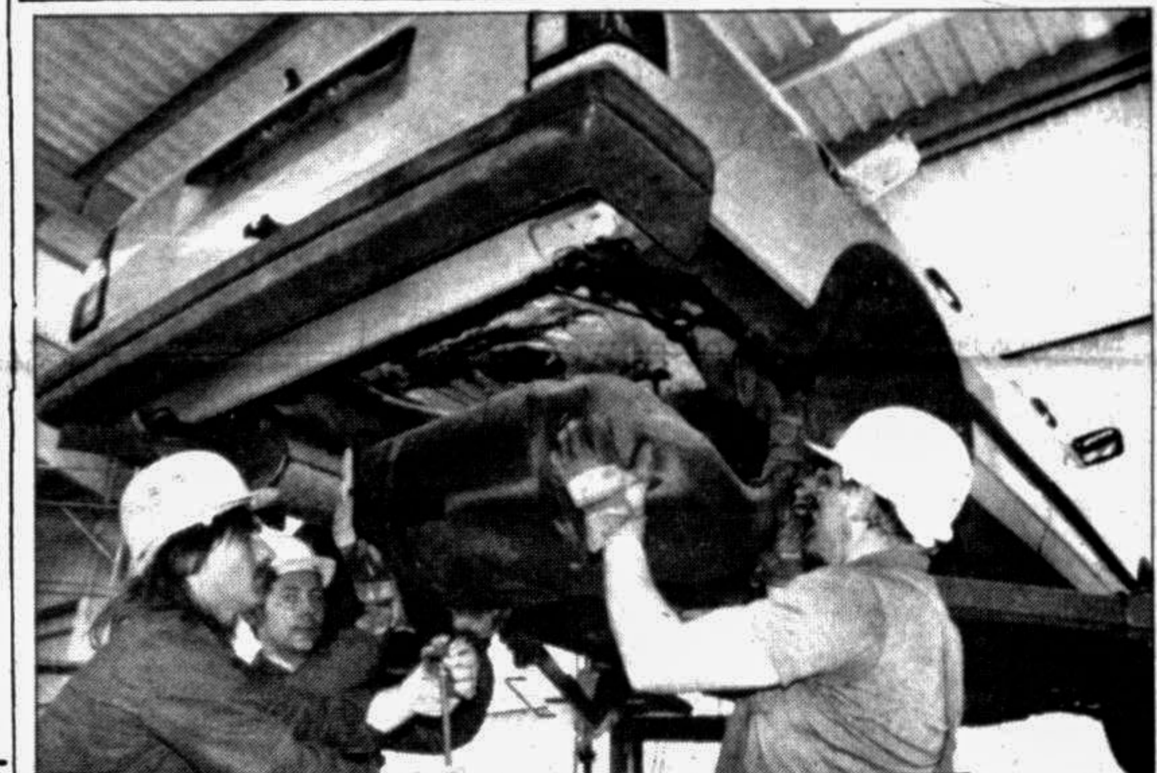
Shown, a pilot plant in northern Germany for the reprocessing of old automobiles: Workers here are removing the gasoline tank from an accident vehicle in a facility in Leer (East Friesland, in Lower Saxony).
