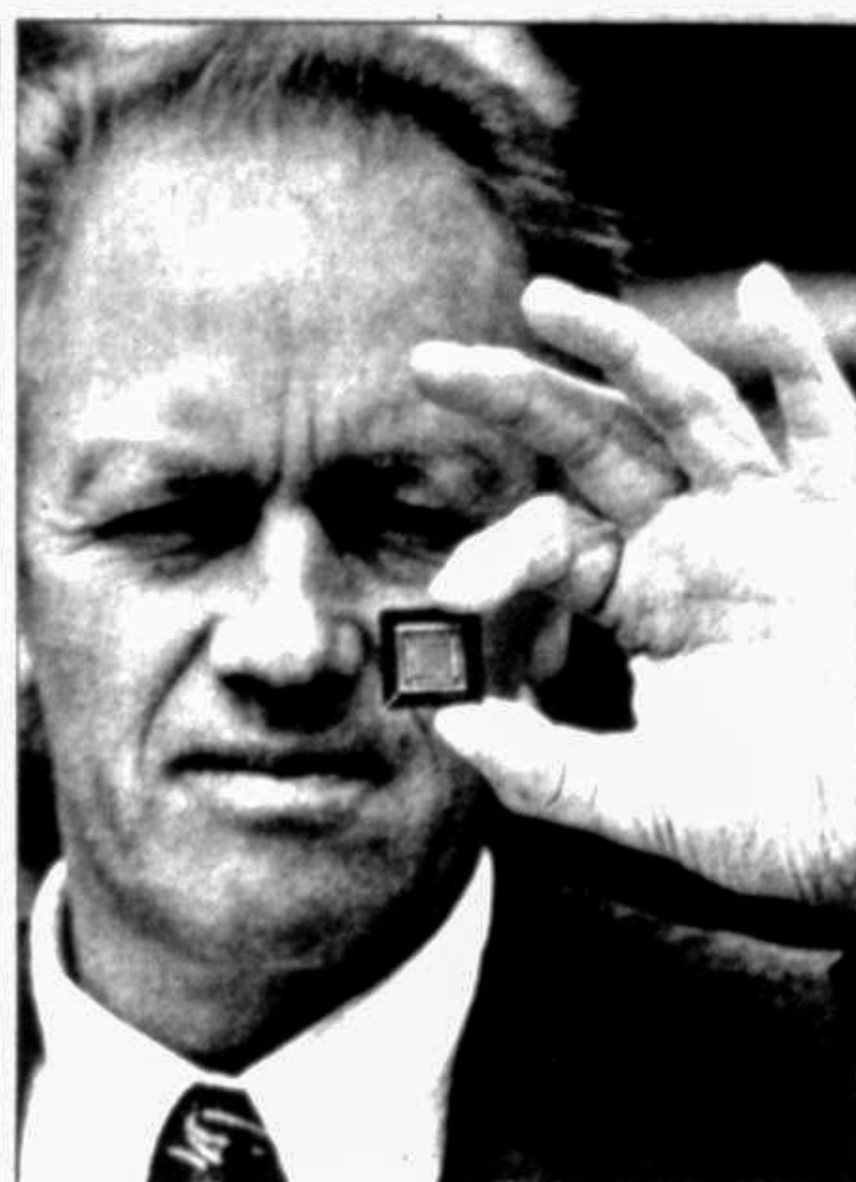
CAMERA ON A SILICON CHIP: This low-power-consuming stamp-sized video camera can be produced for about $25 using world-leading technology developed by research scientists at Edinburgh University, Scotland. Potential applications for the new micro-camera technology include security, machine vision, medical imaging, robotics and consumer products. — LPS photo
