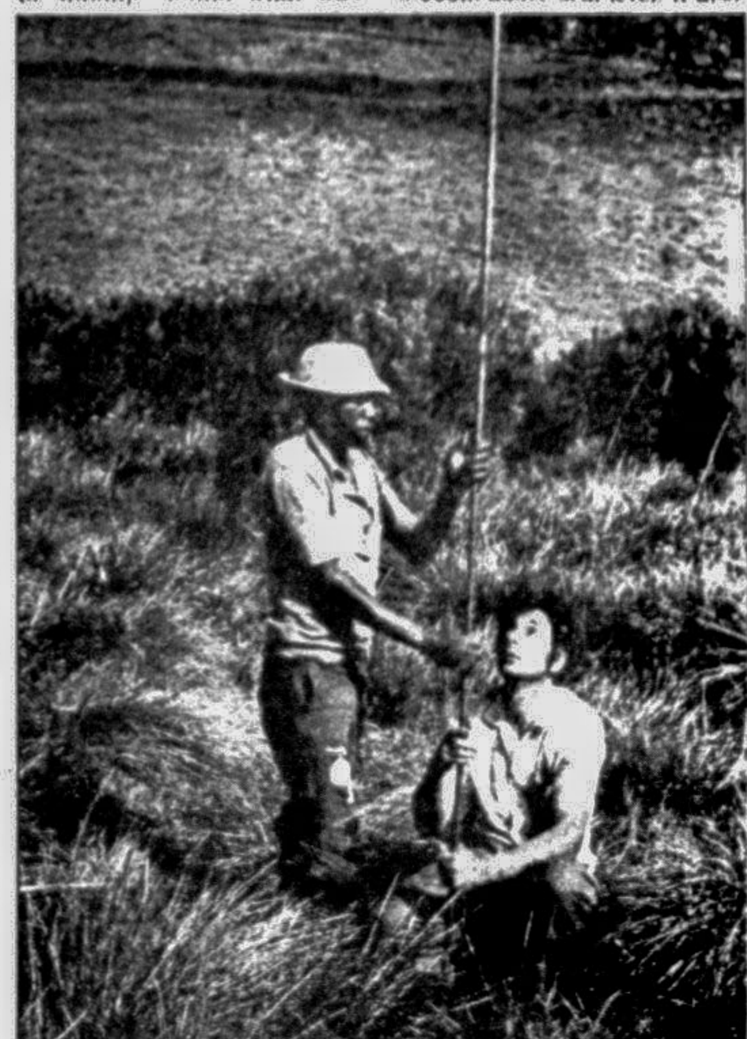
Dr Alan Hamilton, WWF International Plant Conservation Officer (right) at work in the field. Aided by a Ugandan assistant, he is using a probe to sample sediment in order to investigate the past history of vegetation and climate in south-western Uganda.
