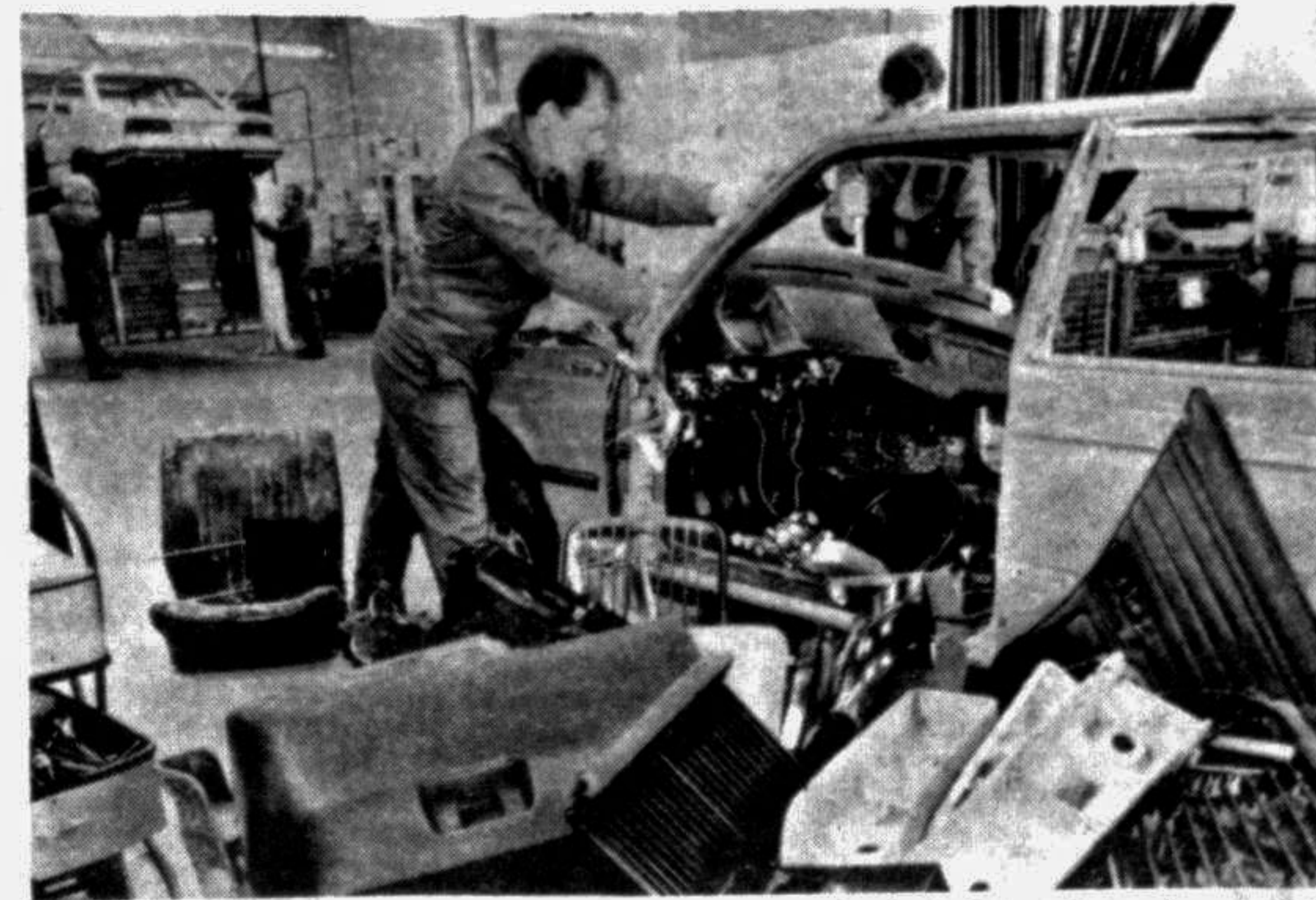
A good measure of the interest of the German automobile industry in environmental protection is provided by this recycling pilot project run by BMW. Successful recycling depends on efficient ways to separate and sort distinct materials in a product. Only then is the cost-effective and meaningful re-use of components assured.
