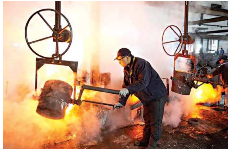
A worker pours molten iron into a mould at a mill manufacturing marine engine components in Huaian, Jiangsu province, China.
