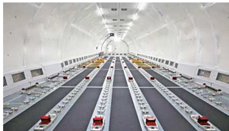
View of the interior of a fully converted Airbus A321 freighter at an ST Engineering hangar in Singapore.
