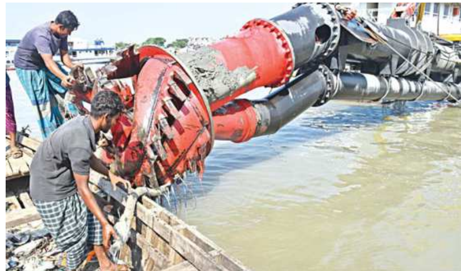
BIWTA staffers separate non-biodegradable waste and silt picked up by dredging machines. This photo was taken on Sunday from the Barishal River Port.
