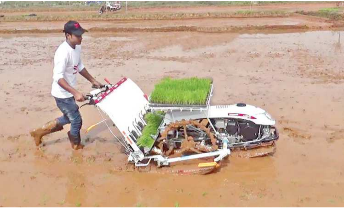
Field demonstration of Yanmar rice transplanter AP4 walking type in Gazipur.
