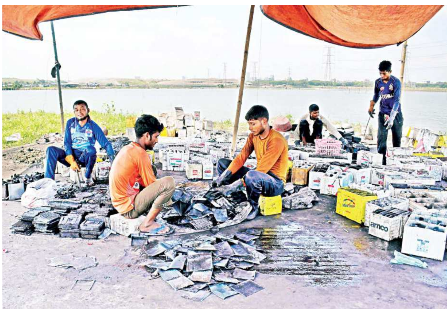
Men taking apart used lead-acid batteries to recycle the parts at an unauthorised and temporary factory in Matuail on the outskirts of the capital. Such factories contribute to the reduction of pollutants in the environment but the business is largely market driven and unregulated.
