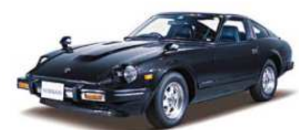
Third Generation Z31 (1984-1989) Two things happened with the new 300ZX. First, Nissan completely dropped Datsun badge, bringing all of their cars under the parent nameplate. Second, the inline six-cylinder was phased out for the 3.0 liter VG30E, Japan’s first mass-
