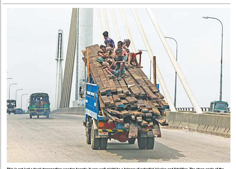
This is not just a truck transporting wooden boards; it very well might be a bringer of potential injuries and fatalities. The steep angle of the tied up boards, the workers sitting on top, the flimsy ropes -- all could be reasons for a terrible accident. One small slip and the men could fall off and get hit by the fast-moving vehicles on Shah Amanat Bridge in Chattogram. A board sliding off could slam into one of the many cars behind. This photo was taken yesterday.
