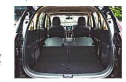
charging needs. For hauling non-human goods, both second and third-row seats can be folded down, giving you a massive 1,608 liter of cargo space. Additional cargo room can also be found under the rear trunk liner, while the tools are hidden under a difficult-to-operate panel on the left D pillar. The rear storage comes at the cost of the spare tire, which has been relocated under the car. You need to undo two bolts in the trunk to access it.
