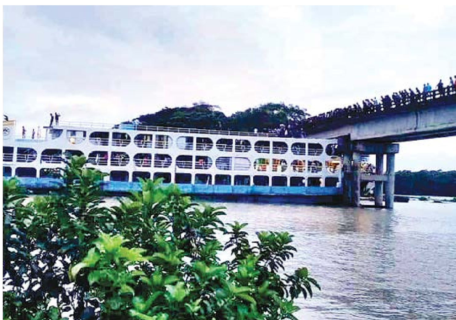
A launch rams the Peyarpur Bridge while trying to go under the structure in Barishal's Bakerganj upazila on Wednesday afternoon. The Pandab river swelled due to rain and water from upstream, reducing the clearance for the bridge. The vessel remained trapped there for nearly five hours until the water receded.
