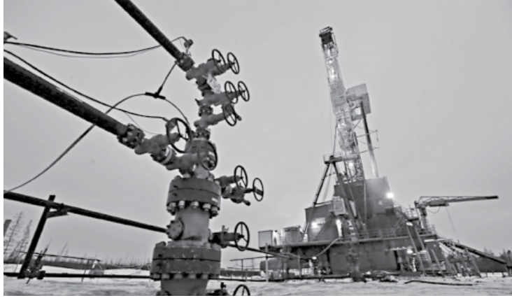
A well head and a drilling rig are seen in the Yarkta Oil Field in Irkutsk Region, Russia.
