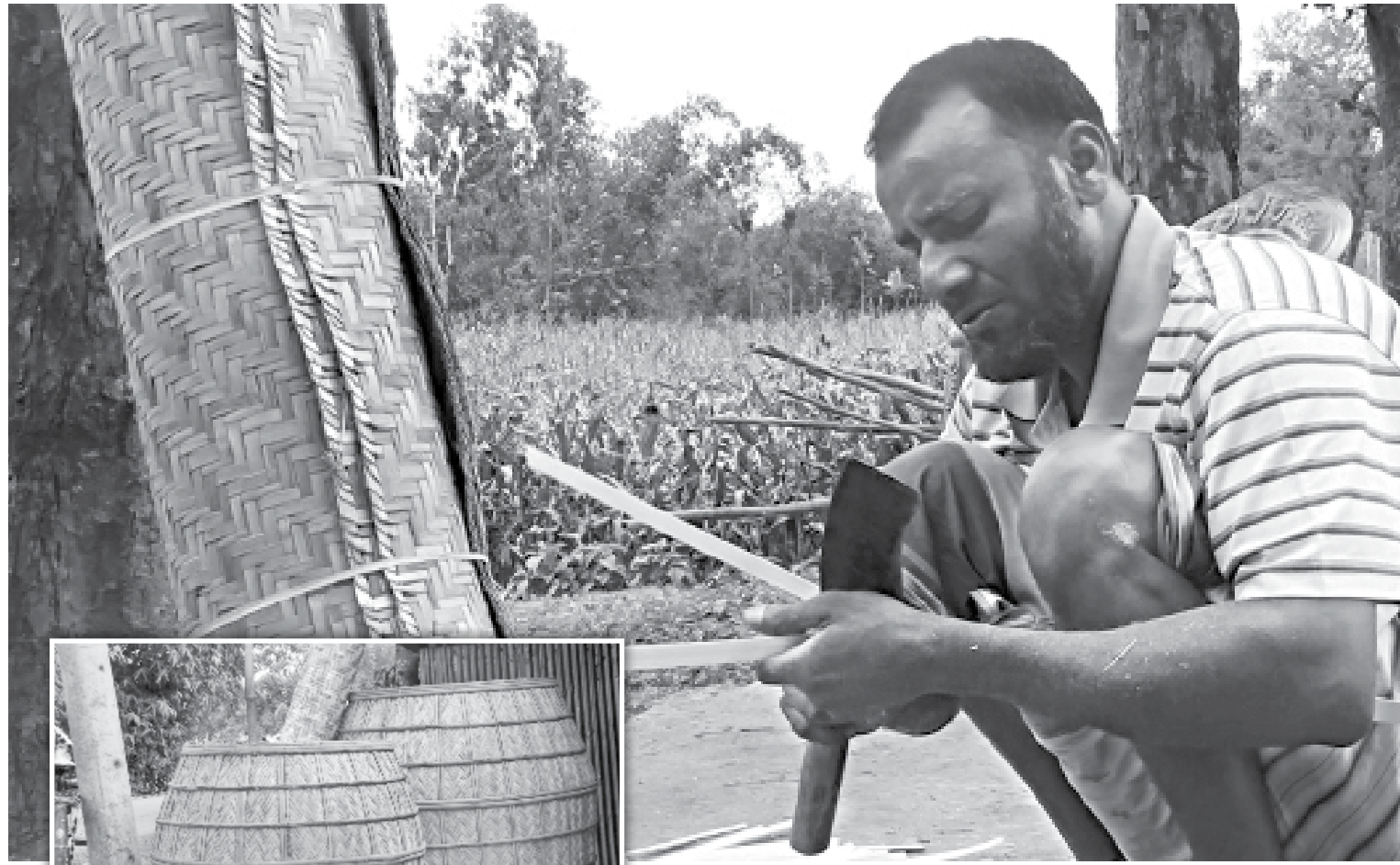
A craftsman in Kamalabari village of Lalmonirhat's Aditmari upazila uses hand tools and slivers of bamboo to make duli, inset, a miniature rice silo that the farmers use to store the grain for consumption by family members till the next harvest.
