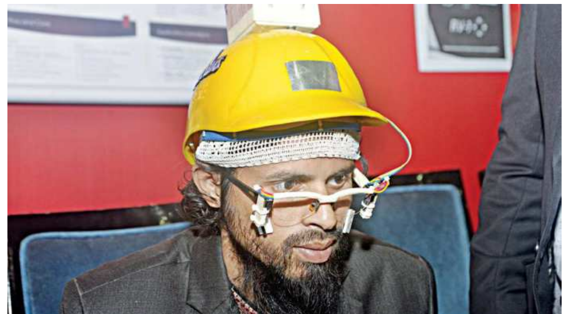
Auxilio lets users use their heads and eyes to control a computer mouse.
