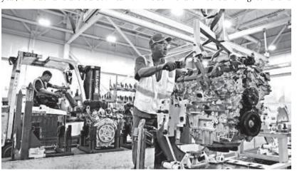
A worker moves a V6 engine, used in a variety of GM cars, trucks and crossovers, from the final assembly line at the GM Romulus Powertrain plant in Michigan, US.
