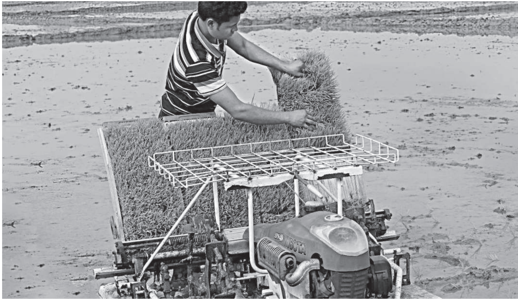
A worker loads a mechanised paddy transplanting machine with seedlings in Chawkerhaat village of Biral upazila. The photo was taken on Tuesday. PHOTO: STAR
