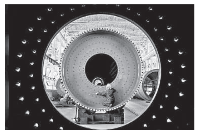
An employee measures a newly manufactured ball mill machine at a factory in China.
