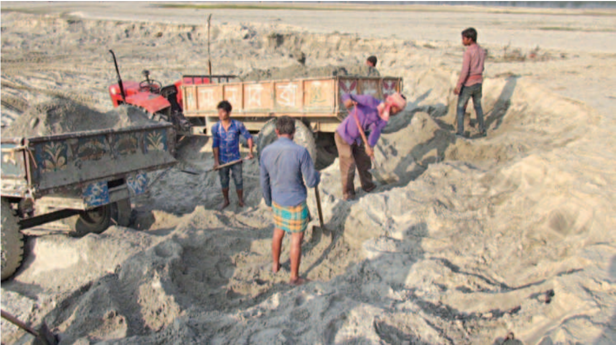
Sand being lifted from the bed of the Dharla river and loaded on to trailers to be carried elsewhere for sale defying a ban. Unregulated sand lifting during the dry season exacerbate erosion of the banks in monsoon.
