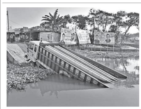
This truck carrying electric poles partially capsized in the Arial Kha river in Barishal yesterday after the pontoon at Mirgani Ferry Ghat could not handle the load. According to officials, the accident took place due to overloading as the truck was supposed to carry 15 poles instead of 30. Road communication from the city to Muladi upazila still remains snapped due to the incident, reports our correspondent.
