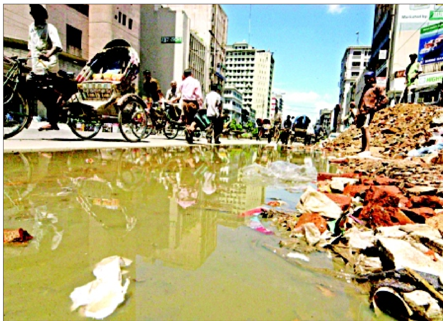
Rubble and construction materials left on the side of a street in Motijheel in the capital clogging the drainage system and creating puddles. This disrupts movement of pedestrians and vehicles and creates a breeding ground for mosquitoes.
