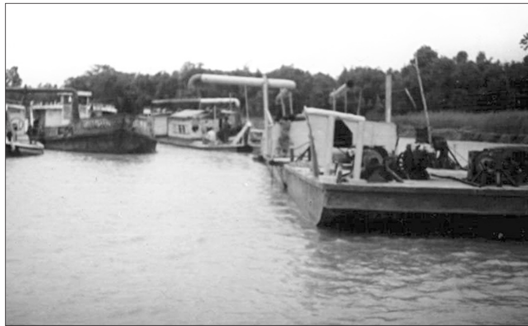
Four dredgers lifting sand from Bongshai river at Jugir Kopha in Mirzapur upazila in Tangail district, accentuating erosion by the river.
