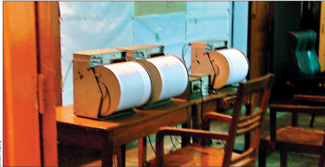
Seismographs used to measure earthquake are seen in the seismic observatory centre at Ambagan.
