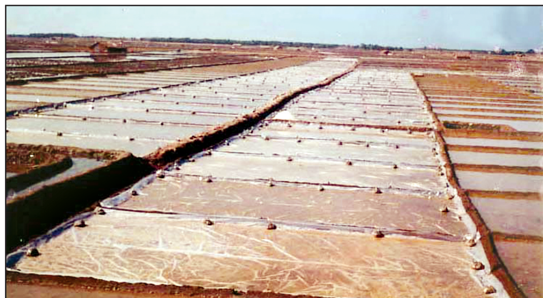
Salt being produced through 'polythene method' in a bed near the beach in Cox's Bazar.
