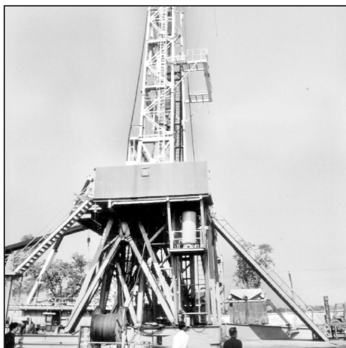
BAPEX drilling Titas-16 gas well in Brahmanbaria
