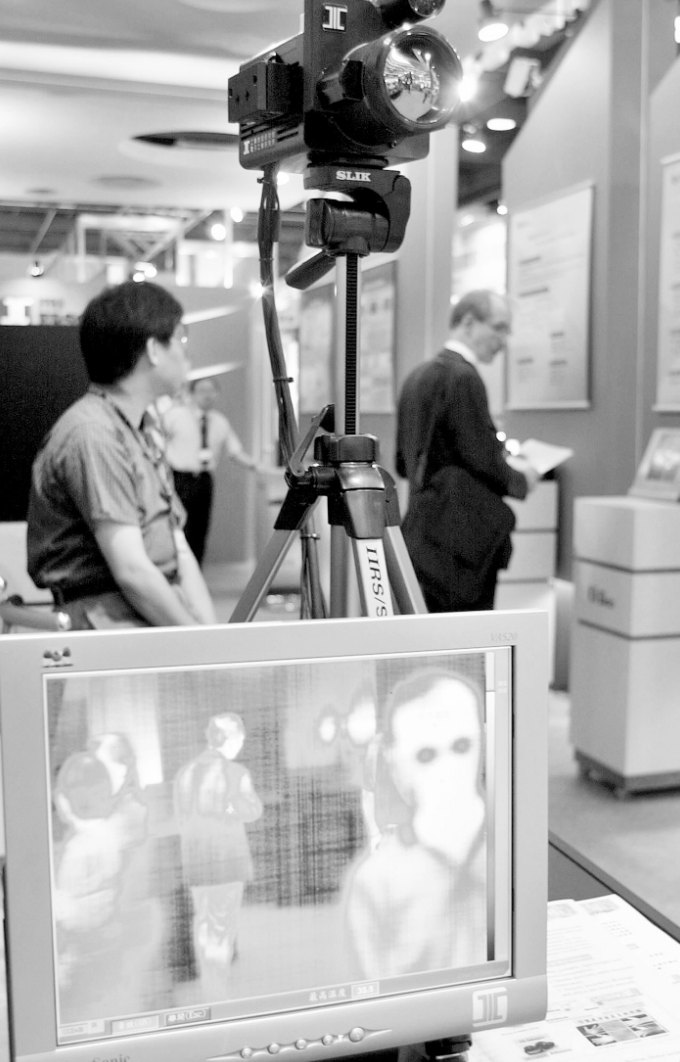
A thermal imaging temperature scanner developed by Taiwan's official Industrial Technology Research Institute is displayed at the four-day electronics equipment and parts exhibition in Taipei on October 12. The portable thermal scanner was widely used in Taiwan when the island was ravaged by Severe Acute Respiratory Syndrome (SARS). Fever was a major symptom shown by SARS patients.
