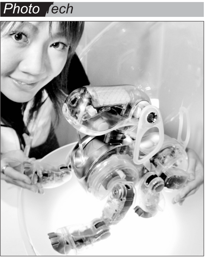
PHOTO: AFP Japan's electronics giant Sony employee Eri Hayakawa displays a skeleton model of the new robot dog 'AIBO ERS-7' during the press preview at the company's showroom in Tokyo on September 26. The new AIBO, weighing 1.6kg, is equipped with 20 joints to make smooth body movements and 576MHz 64bit RISC processor on its CPU. Sony will put it on the market in November with a price of 185,000 yen (1,580 USD).
