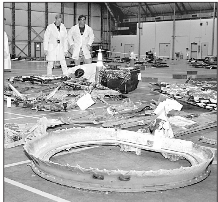
Members of the Columbia Reconstruction Team examine pieces of debris in the RLV hanger at Kennedy Space Centre, FL. Over three thousand pieces have arrived and more debris is arriving every several days from Louisiana and Texas for cataloguing, layout and examination.
